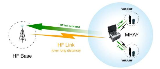
**MRAY Solution**: The field personnel deploy an MRAY transportable radio and use the HF link to communicate back to the command center. The command center can use an HF radio (or an MRAY) to create a link to the field personnel (via the MRAY) over long distance. The field personnel do not require HF radio equipment to communicate back with the command center, using less expensive and smaller LMR handheld radios.
