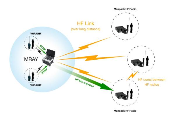
**MRAY Solution**: An MRAY transportable radio system is used to create a local communications area with LMR equipment while crosspatching to HF in order to extend long distance communications to other field personnel using HF "manpack" radios. The HF radios can also communicate directly with each other over HF radio links created from manpack to manpack.
